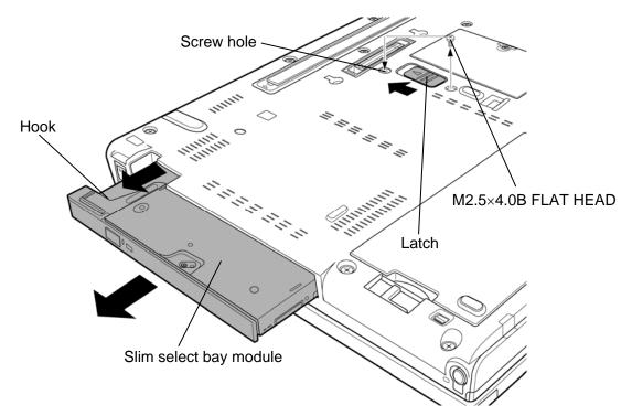
Figure 4-9 Removing the slim select bay module
